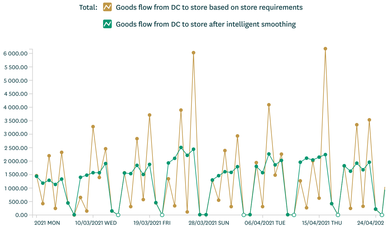
Figure 8: Orange line = goods flow from distribution center to store based on store inventory requirements; green line = goods flow from distribution center to store when intelligent delivery flow smoothing is applied.
